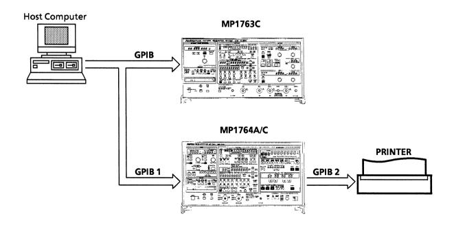
By means of controlling MP1763C and MP1764A/C using the host computer via GPIB 1 port, data can be output to the printer via MP1764A/C GPIB 2 port.
