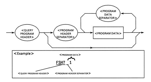
For both <COMMAND MESSAGE UNITS> and <QUERY MESSAGE UNITS>, a space must be inserted between the program header and any program data immediately following it. The application, function and operation of the program data can be seen from the program header. If there is no program data; the application, function or operation to be performed by a device is indicated by the header alone.
