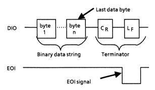
EOI ON / OFF is one statement for controlling the EOI line. The default is EOI OFF which means that the EOI line is not controlled. Specifying EOI ON causes an EOI signal to be transmitted at the same time as terminator LF when the last data byte of the WRITE@ statement is transmitted.
