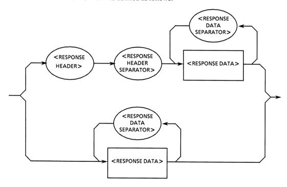
A <RESPONSE MESSAGE UNIT > consists of 2 basic types of syntax. The first is a response message with a header which returns the results of processing data on settings made by program messages. The second is a response message unit without a header which returns only measured results.
