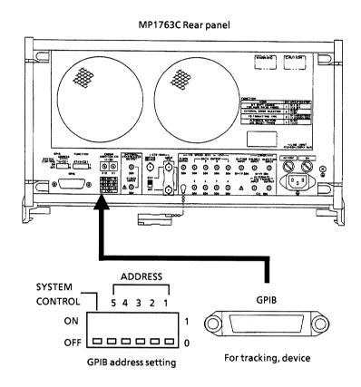
The GPIB address can be set 0 to 30. Five switches are weighed differently: "5", "4", "3", "2" and "1" are respectively weighed to 16, 8, 4, 2 and 1.
