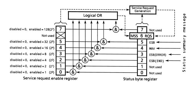
The table below shows the conditions for the MP1763C's status byte register.
