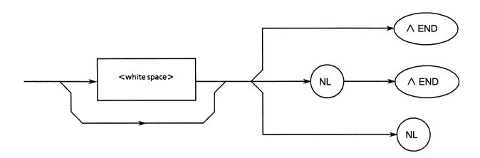
A <PROGRAM MESSAGE TERMINATOR> terminates a sequence of one or more <PROGRAM MESSAGE UNIT> elements of a fixed length.
