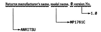
If an \*IDN? common query is sent to a device when the manufacturer is Anritsu, the model is MP1763C, and the firmware version is 1; a response message comprising the four fields shown above is returned.
