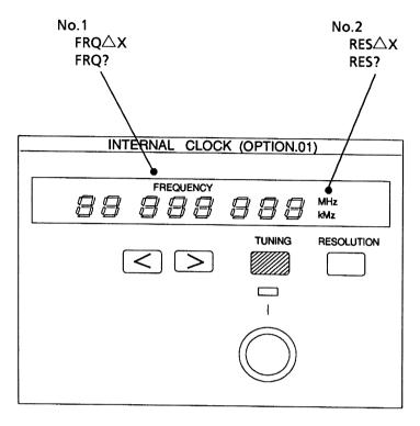
Fig. 9-2-(1) INTERNAL CLOCK Section
