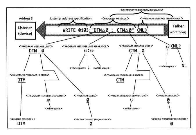
The program message format is a sequence of functional elements which are the minimum requirement for indicating a function. The groups of upper-case alphabetic characters enclosed by <> in the diagram above are examples of functional elements. Functional elements can be further divided into "encoded elements". The groups of lower-case alphabetic characters enclosed by <> in the diagram above are examples of encoded elements.
