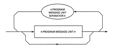
A <PROGRAM MESSAGE > consists of zeros, or a sequence of one or several <PROGRAM MESSAGE UNIT > elements. <PROGRAM MESSAGE UNIT > elements are either programming commands or data sent from the controller to devices. The <PROGRAM MESSAGE UNIT SEPARATOR > element is used to separate <PROGRAM MESSAGE UNITS >.
