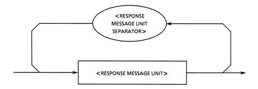
A <RESPONSE MESSAGE > consists of one <RESPONSE MESSAGE UNIT > element or a sequence of many <RESPONSE MESSAGE UNIT > elements. A <RESPONSE MESSAGE UNIT > element is a single message sent from a device to the controller. A <RESPONSE MESSAGE UNIT SEPARATOR > element is used to separate <RESPONSE MESSAGE UNIT > elements.
