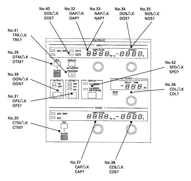
Fig. 9-2-(4) OUTPUT Section
