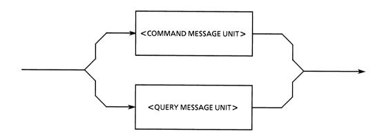
A <PROGRAM MESSAGE UNIT> is either the <COMMAND MESSAGE UNIT> or <QUERY MESSAGE UNIT> received by a device. <COMMAND MESSAGE UNITS> and <QUERY MESSAGE UNITS> are explained in detail on the next page.
