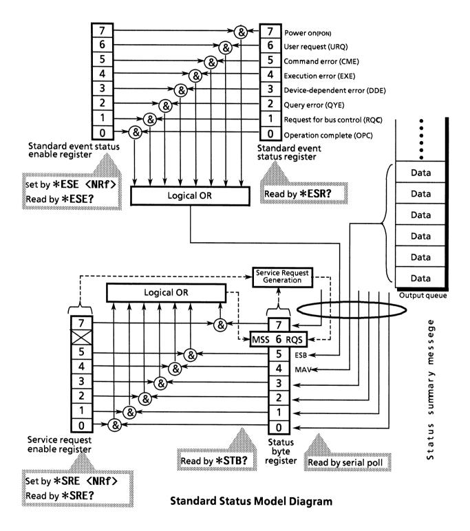
The IEEE 488.1 status byte is used in the status model. This status byte is composed of 7 summary message bits given from the status data structure. For creating the summary message bits, there are 2 models for the data structure - the register model and the queue model.
