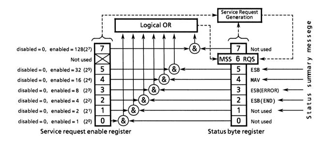
**\*SRE?** Service Request Enable Query (Returns the current value of the service request enable register)
