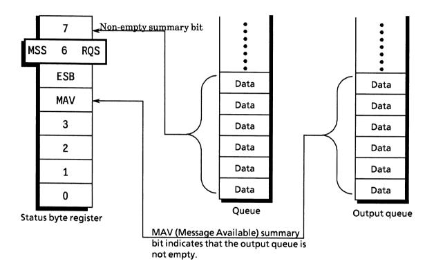
The output queue, which is mandatory, is the queue that outputs the MAV summary message to bit 4 of the status byte. A queue (which can output the MAV summary message to any of bits 0 to 3 or 7 of the status byte register) is an option and is simply called a "queue".
