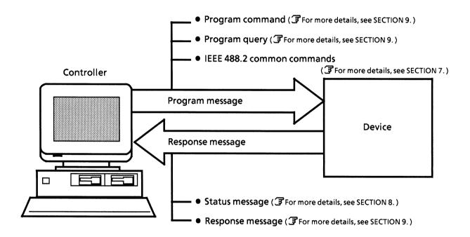
The messages described above are transferred via the input and output buffers of the device. The output buffer is also referred to as an output queue. The following table gives a brief explanation of input and output buffers.
